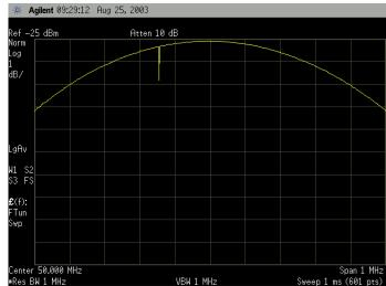
Effected instruments will randomly show an amplitude drop of approximately 2 to 3 dB.
